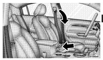
Inserting Latch Plate into Buckle
